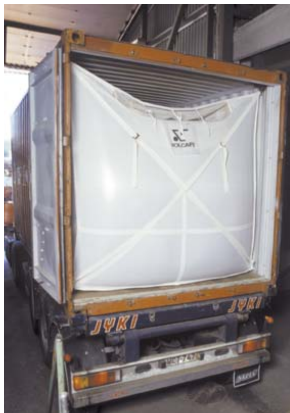
Large-size in-lets that fill an entire container have replaced the smaller jute bags, reducing waste.
